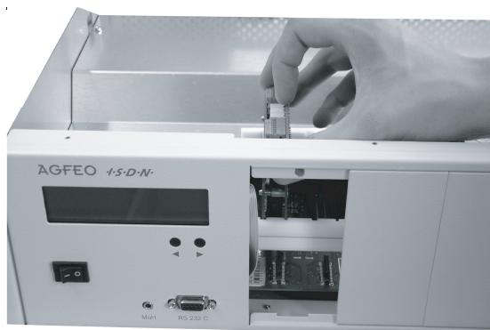
Slide the modules into the guide and press down until they fit securely into the slot.
