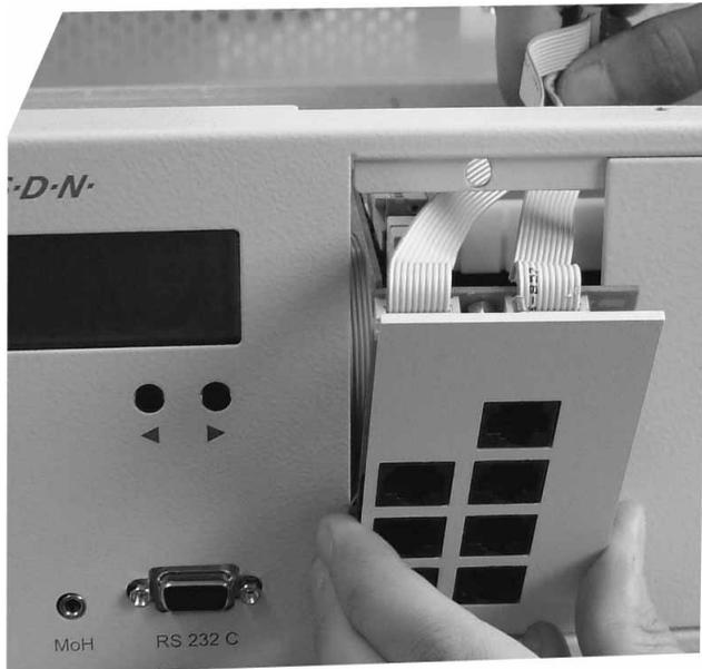
To insert the front plate, hook the notch on the bottom edge into the appropriate groove. Push the cable through the opening in the front plate as shown in the photograph. Then shut the front plate and screw it tight using the knurled screws.
